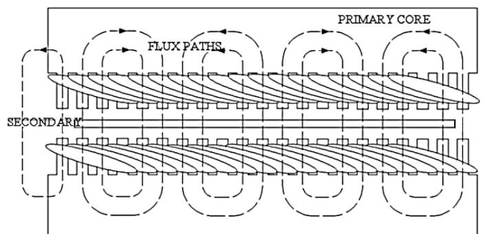
Figure 2. Flux paths in a double sided linear induction motor
