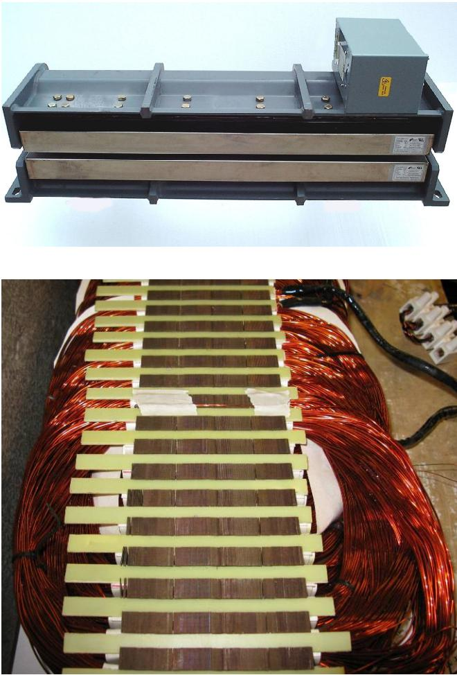
Figure 3. Double sided stator launch assembly
