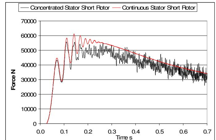
Figure 10. Force-time curve for offset launcher
